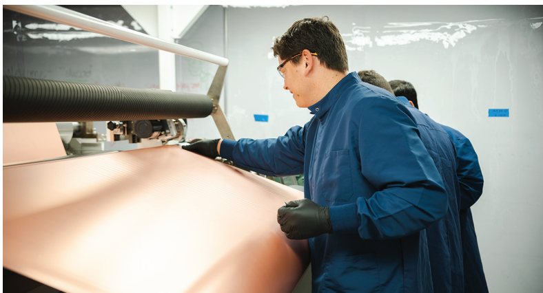
Copper foil inspection Photo courtesy of Redwood Materials
