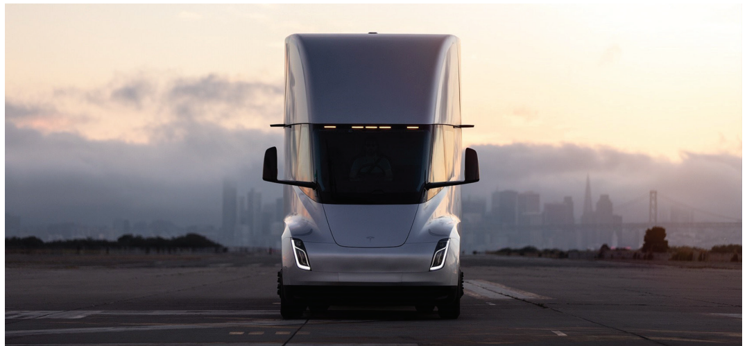
The Semi truck coming from Tesla and attracting interest since 2020 from such buyers as Walmart Canada is said to have 500 miles of range and energy consumption of less than 2 kilowatt-hours per mile. Image courtesy of Tesla and Walmart Canada
